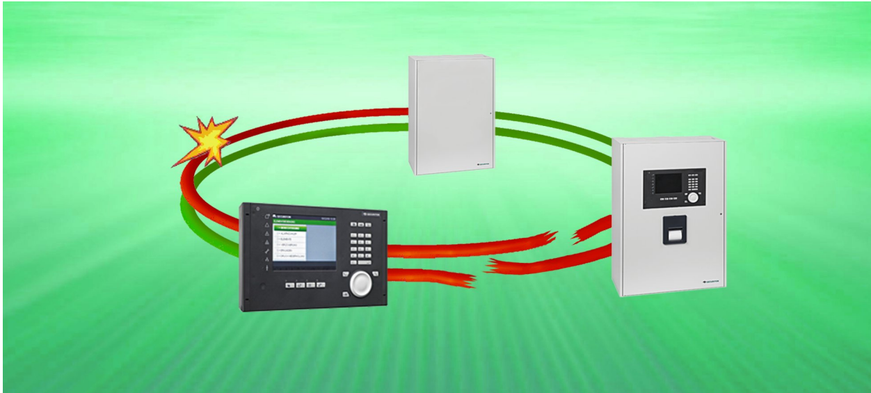
Fig. 7 Redundant design of a SecuriLan
