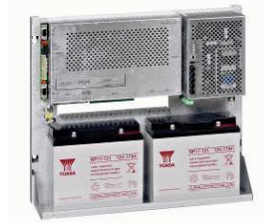
Fig. 20 Module cover and rechargeable cells
